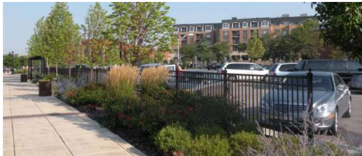
Landscape screening along surface parking lots. These areas can also accommodate storm water runoff from sidewalks and parking lots.
